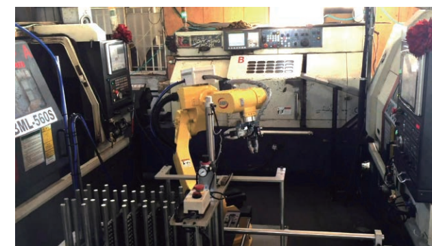
CNC加工機上下料(1對3車床) 1 to 3 CNC loading and unloading
