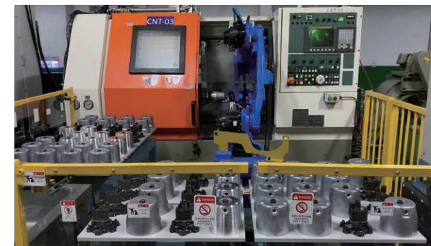
CNC加工機上下料(1對1車床) 1 to 1 CNC loading and unloading
