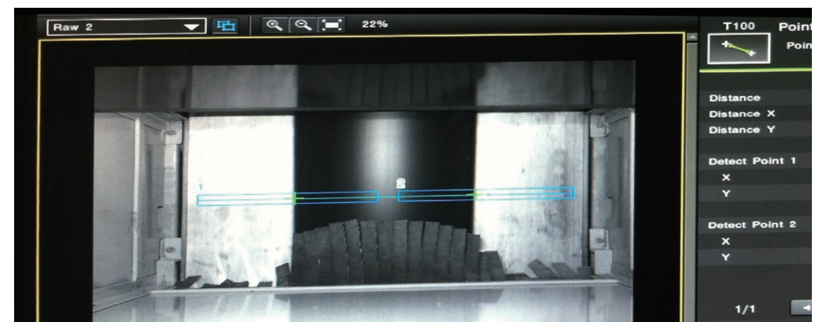
輪胎內胎尺寸量測 Size measurement of tire inner tube
