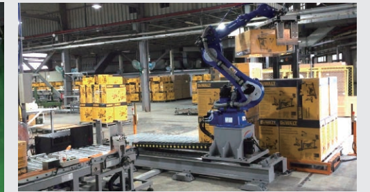
Robot橫移平台(1對4棧板堆疊系統) The 7th axis of the robot-traverse platform
