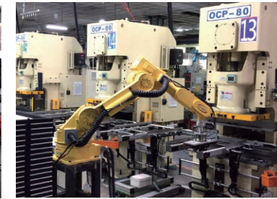
高速精密沖床上下料 Loading and unloading of high-speed precision punch machines
