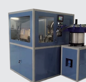
客製化設備-全自動金屬加工品視覺檢測 Automatic visual inspections of metal products
