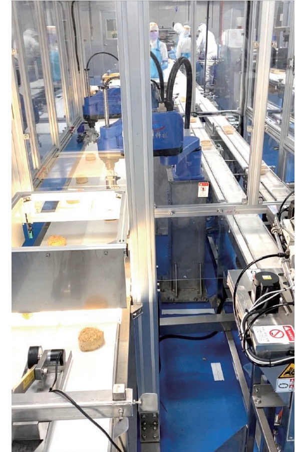
冷凍飯糰定位辨識 Positioning identification of frozen rice balls
