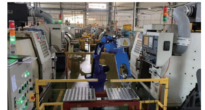
CNC加工機上下料(1對2車床) 1 to 2 CNC loading and unloading
