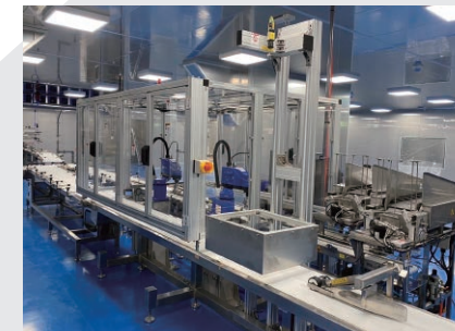
全自動影像辨識機械手臂動態抓取入Tray盒 Automatic visual inspections and SCARA dynamic grabbing into the tray
