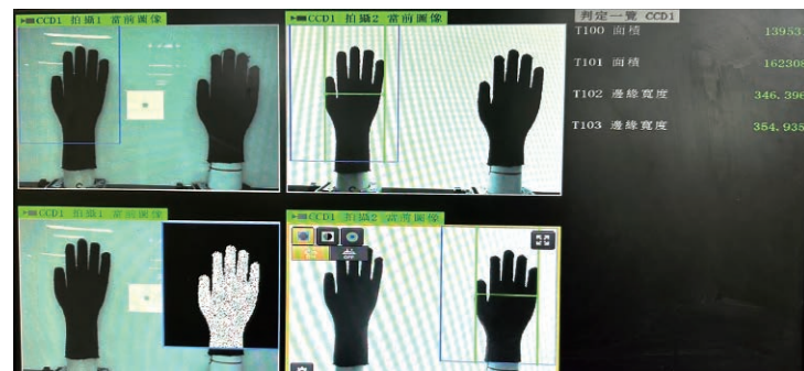
手套尺寸辨識 Glove size identification
